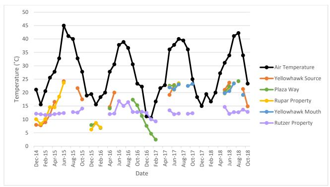
Figure 4. Maximum air temperature compared to maximum stream temperature for Yellowhawk Creek sites. Monthly maximum stream temperatures at Yellowhawk Creek monitoring sites were graphed against monthly average Walla Walla air temperature displayed in black over the same time.
