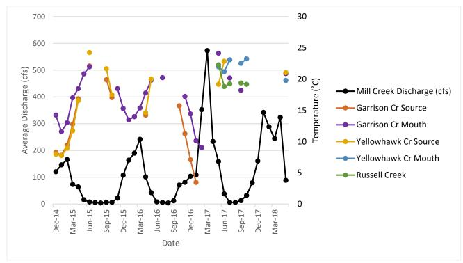
Figure 15. Monthly average Mill Creek discharge compared to maximum stream temperature at all distributary sites. Monthly maximum stream temperatures for all distributary monitoring sites were graphed against monthly average Mill Creek discharge displayed in black across the same time.
