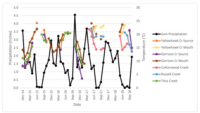
Figure 7. Total monthly precipitation compared to maximum stream temperature at all distributary sites. Monthly maximum stream temperatures from all distributary monitoring sites were graphed against the monthly sum precipitation in Walla Walla displayed in black across the same time.
