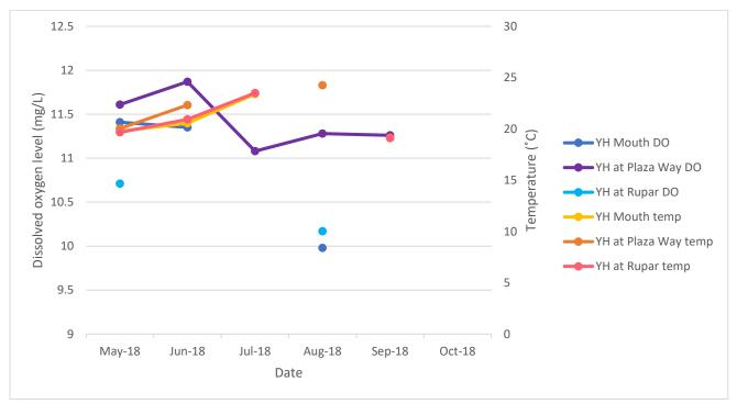
Figure 13. Maximum dissolved oxygen levels compared to maximum stream temperature at three Yellowhawk Creek sites in 2018. Monthly maximum dissolved oxygen levels are displayed in cooler colors (blues and purple) while the maximum stream temperatures are displayed in warmer colors (yellow, orange, and pink). These three sites represent Yellowhawk at the Mouth, Yellowhawk at Plaza Way, and Yellowhawk on Rupar Property.
