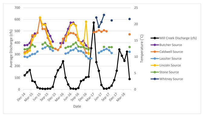
Figure 14. Monthly average Mill Creek discharge compared to maximum stream temperature at spring creek source sites. Monthly maximum stream temperatures from spring creek source monitoring sites were graphed against monthly average Mill Creek discharge displayed in black across the same time.
