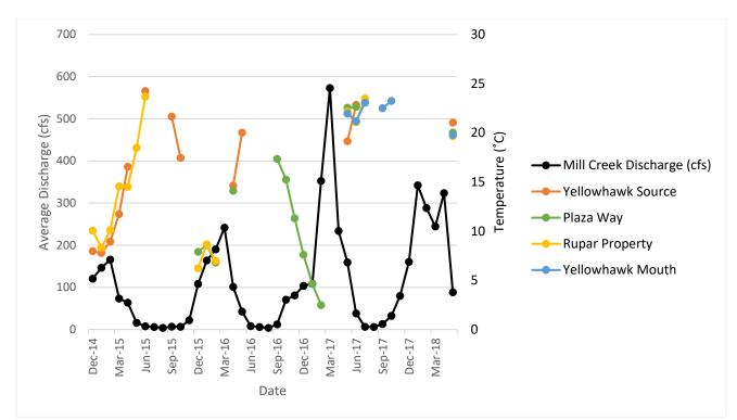
Figure 16. Monthly average Mill Creek Discharge compared to maximum stream temperature at Yellowhawk Creek sites. Monthly maximum stream temperatures at all Yellowhawk Creek monitoring sites were graphed against monthly average Mill Creek discharge displayed in black across the same time.
