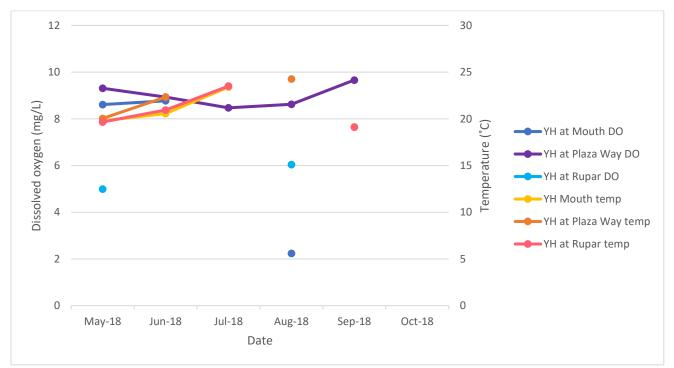
Figure 11. Minimum dissolved oxygen levels compared to maximum stream temperature at three Yellowhawk Creek sites in 2018. Monthly minimum dissolved oxygen levels are displayed in cooler colors (blues and purple) while the maximum stream temperatures are displayed in warmer colors (yellow, orange, and pink). These three sites represent Yellowhawk at the Mouth, Yellowhawk at Plaza Way, and Yellowhawk on Rupar Property.
