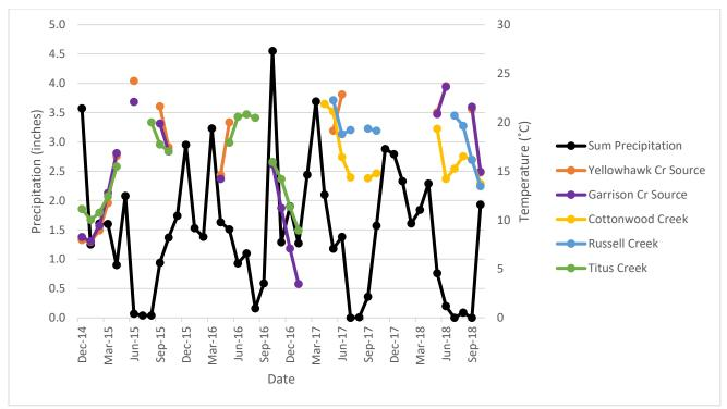
Figure 8. Total monthly precipitation compared to maximum stream temperature at distributary source sites. Monthly maximum stream temperatures from distributary source monitoring sites were graphed against the monthly total precipitation in Walla Walla displayed in black across the same time.
