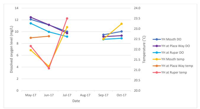
Figure 12. Maximum dissolved oxygen levels compared to maximum stream temperature at three Yellowhawk Creek sites in 2017. Monthly maximum dissolved oxygen levels are displayed in cooler colors (blues and purple) while the maximum stream temperatures are displayed in warmer colors (yellow, orange, and pink). These three sites represent Yellowhawk at the Mouth, Yellowhawk at Plaza Way, and Yellowhawk on Rupar Property.
